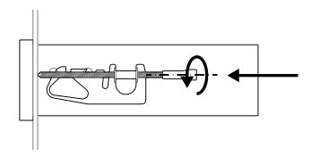
4. Turn the set screw with a blade screwdriver to the stop on the front plate.
