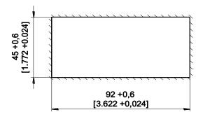
Cutout according to DIN 43700 Maximum material thickness: 5 mm [.197]
