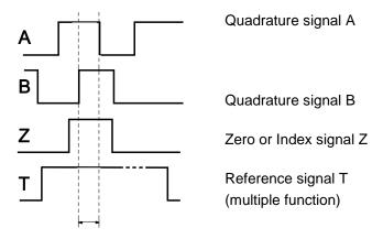
The reset of the display takes place for the condition (A & B & Z) resp. (A & B & Z & T).
